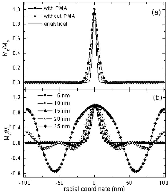
Fig. 3. (a) Line scan of the out-of-plane magnetization component  $M_z$  across the diameter ( $t = 5$  nm,  $\phi = 60$  nm) for three different cases as discussed in the text. (b)  $M_z$  line scan profiles across the diameter as a function of dot thickness for  $\phi = 200$  nm in the case of epitaxial dots with PMA.
