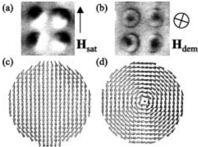
Fig. 1. MFM images ( $0.8 \mu\text{m} \times 0.8 \mu\text{m}$ ) corresponding to (a) an in-plane remanent state and (b) an out-of-plane demagnetized state for dots of  $t = 10 \text{ nm}$  and  $\phi = 200 \text{ nm}$ . Top view of (c) a single domain and (d) a vortex-like state obtained from 3D micromagnetic calculations.
