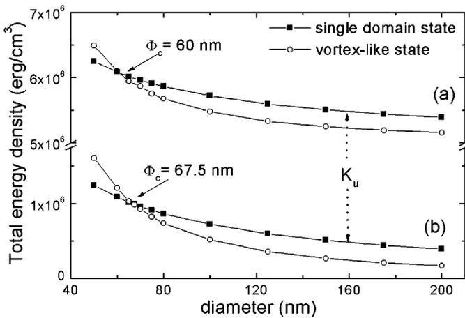
Fig. 2. The total free energy density of the V and SD state as a function of the dot diameter for  $t = 5 \text{ nm}$  and for dots (a) with  $K_u = 5 \times 10^6 \text{ erg/cm}^3$  and (b) with  $K_u = 0$ .
