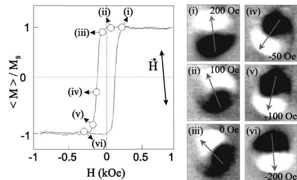
FIG. 3. Reversal of the magnetization by coherent rotation for a 10-nm-thick and 500-nm-large dot. The MFM images (i)–(vi) display the magnetic contrast corresponding to the distribution of the magnetization at different applied field values.
