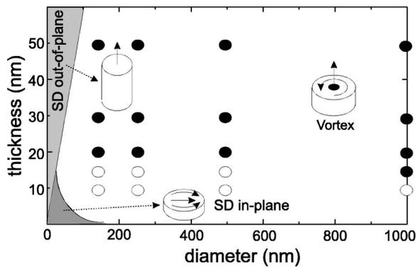
FIG. 1. Calculated ground state diagram for polycrystalline Co dots. The experimental points obtained from the hysteresis loops are indicated by open circles for a reversal yielding square hysteresis loops, respectively, by full circles for a reversal through vortex formation.
