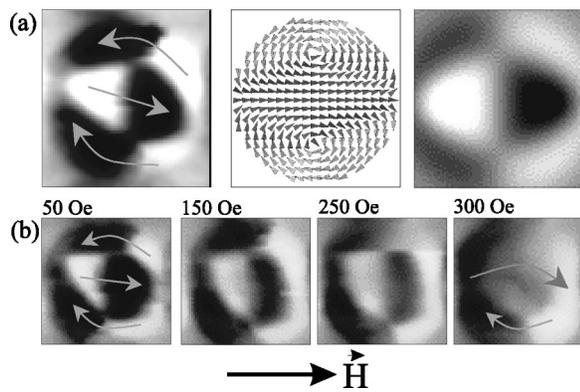
FIG. 4. (a) On the left, the MFM contrast corresponds to a double vortex state, observed in a 30-nm-thick and 1000-nm-large dot. In the center the simulated micromagnetic configuration is shown. On the right, the gray scale representation of the calculated divergence of the magnetization distribution corresponds to the micromagnetic configuration. (b) MFM images series under applied field showing the expulsion of one vortex.
