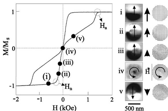
FIG. 2. Reversal of the magnetization through vortex formation for a 30-nm-thick and 500-nm-diam dot. Different points on the hysteresis curve, from (i) to (iv), are visualized by MFM.
