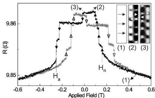
Fig. 2. The MR response of a 90 nm thick and 100 nm wide wire, at room temperature. Full circles and full line: the field is decreased from positive saturation (point (1)). Different stages along the cycle, after the nucleation of the walls ( $H_n$ ) are illustrated by the MFM images (2) and (3). At the annihilation field ( $H_a$ ), the walls are completely erased.
