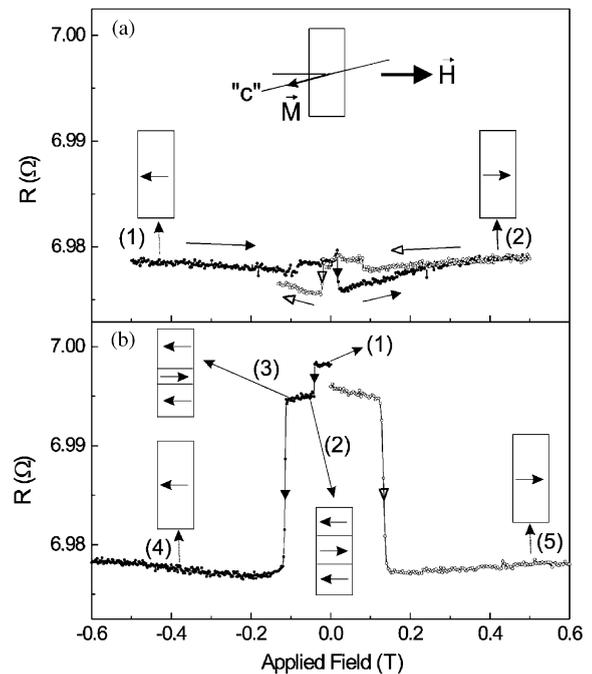
Fig. 3. (a) The MR hysteresis cycle of a 30 nm thick and 300 nm wide wire at 10 K. A schematic of the misalignment of the easy axis with respect to the normal to the wire axis. (b) MR curve corresponding to the remagnetization in a negative field (full circles) or in a positive field (open circles) applied perpendicular to the wire axis, after saturation in a field parallel to the wire axis.
